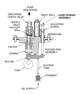
lubricant from the reservoir to be drawn into the well until pressure is equalized. On the piston upstroke, the oil in the piston cylinder reseats the inlet shutoff ball and is forced out through the discharge check valve to the machine injection point.
