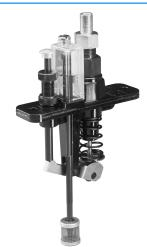
is created in the area between the piston and the discharge check valve. The supply inlet shutoff ball is concurrently unseated and lubricant is drawn into the piston cylinder from the sight well. This action creates a pressure reduction (vacuum) in the air- tight sight well, causing
