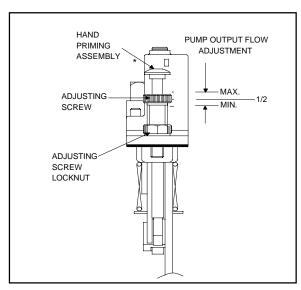
\*Should not reciprocate up and down as pump operates, on pumps built beginning in January 1997.
